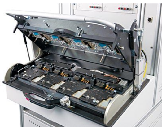
Automotive infotainment test system for testing four infotainment modules simultaneously
