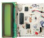
Microcontroller Based Speedometer-cum-Odometer
