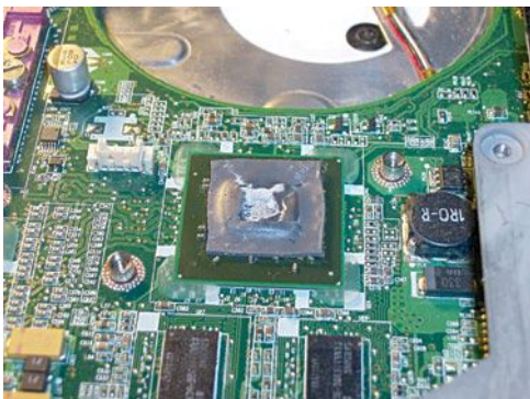
Fig. 2: Thermal pad and paste after prolonged usage
